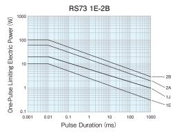
The maximum applicable voltage is equal to the max. overload voltage. Please ask us about the resistance characteristic of continuous applied pulse. The pulse endurance values are not assured values, so be sure to check the products on actual equipment when you use them.
